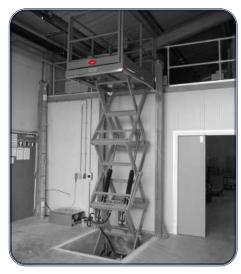
The lifting tables can be adapted to exactly fit your needs. This table has been mounted in a pit for easy access to platform.
